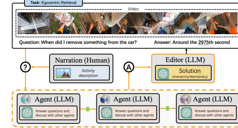
Figure 8: The structure behind the mindstorm occurring in our NLSOM for egocentric retrieval. Several debaters engage with each other in a free-form manner. For more details, see Appendix H.
